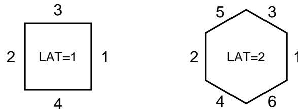
Figure 4.39: Unit structure of lattice.
