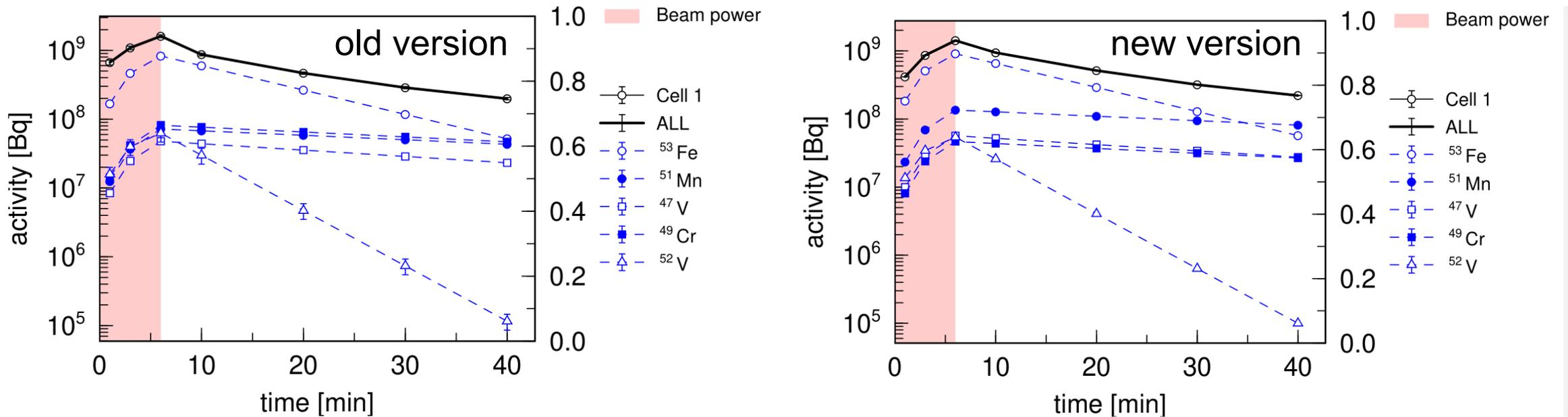
Time dependence of induced activities in Fe target irradiated by 150 MeV protons
