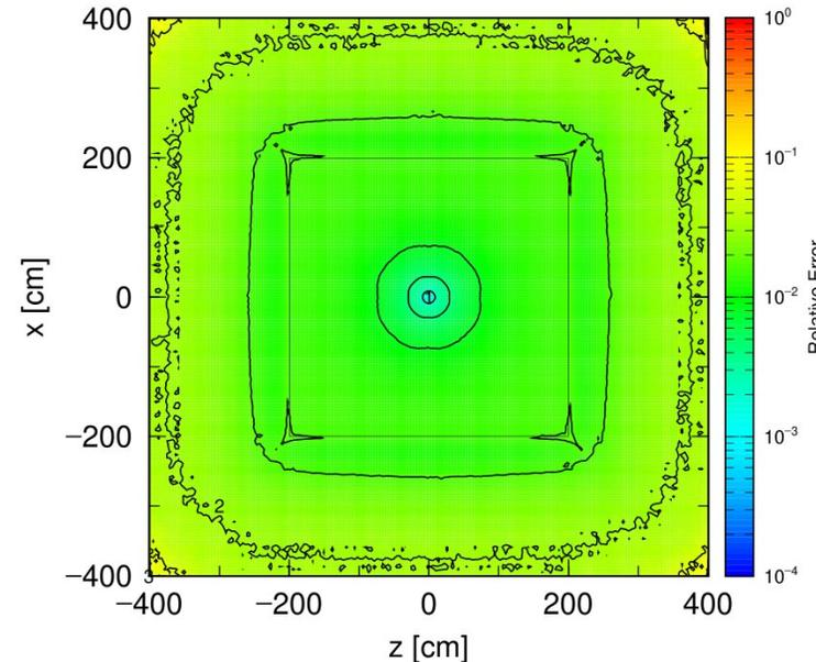
Relative error distributions with and without particle navigation function to the left side
